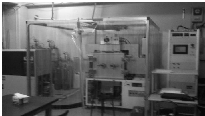
Figure 1 RF-Sputtering system for DLC coating.
