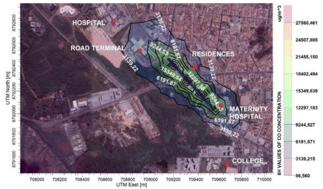
Figure 2. Modelling of 8 hours of CO concentration by using AERMOD dispersion model in the city of Aracaju (Macêdo & Ramos, 2020)
