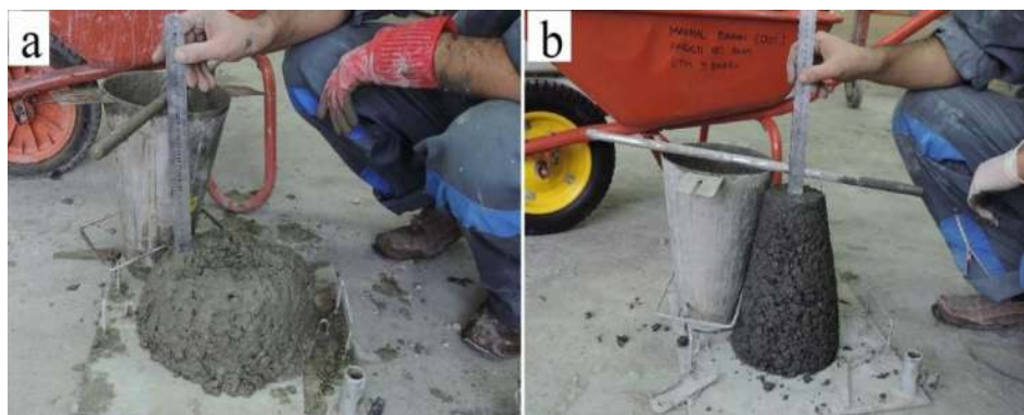
Figure 3. The slump test of (a) plain OPC mix, and (b) POFA-based mix reinforced with WMP fibres.
