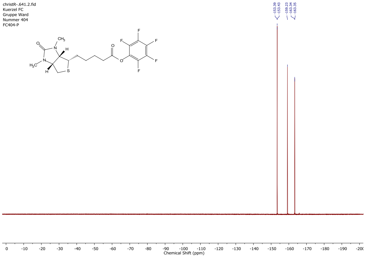
Spectrum 48 19 F NMR Spectrum of Me 2 BiotPFP in DMSO- d 6 .
