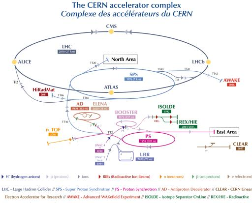
Experiment/High Intensity and Energy ISOLDE // LEIR - Low Energy Ion Ring // LINAC - LINear ACcelerator // n\_TOF - Neutrons Time Of Flight // HiRadMat - High-Radiation to Materials
