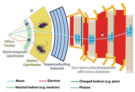
Figure 4.2: A cross-sectional-slice view of the CMS detector illustrating the interactions of various particle types with different detector components [40].
