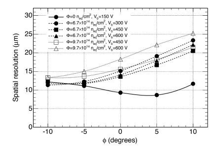
Figure 4.5: Spatial resolution of the pixel along the  $r - \phi$  direction as a function of the angle between the track direction and the normal to the sensor plane [38].
