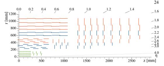
Figure 4.4: Diagram of the CMS inner tracker in one r-z quadrant, with the collision point at the origin. Green lines depict the pixel detector, while the single-sided and double-sided strip trackers are shown in red and blue, respectively [45].
