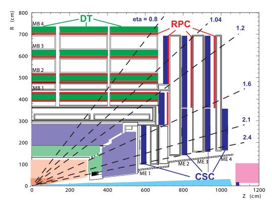
Figure 4.11: Layout of the CMS muon system in one r-z quadrant [38].
