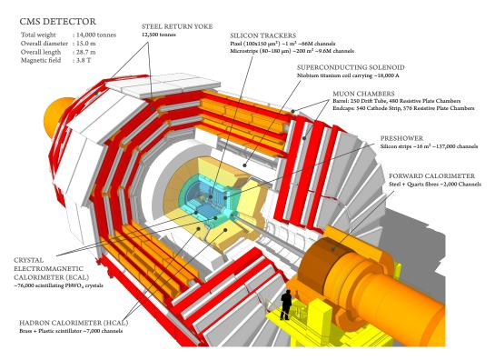
Figure 4.1: Cutway diagrams of the CMS detector [39].
