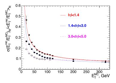
Figure 4.10: The transverse energy resolution as a function of the simulated jet transverse energy for barrel jets ( $|\eta| < 1.4$ ), endcap jets ( $1.4 < |\eta| < 3.0$ ), and forward jets ( $3.0 < |\eta| < 5.0$ ) [38].
