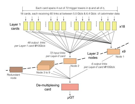
Figure 4.14: The time-multiplexed architecture of the upgraded calorimeter trigger in L1 trigger [53].
