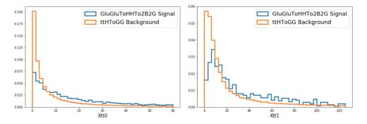
Figure 5.7:  $\chi_t^2$  variables in training to reject events with a hadronic-decay W boson, for events with at least 2 additional jets (left) and 4 additional jets (right) besides the two b jets.
