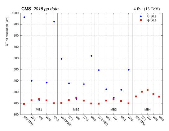
Figure 4.12: The spatial resolution for DT hits in  $\phi$  superlayers (squares) and  $\theta$  superlayers (diamonds) [52].
