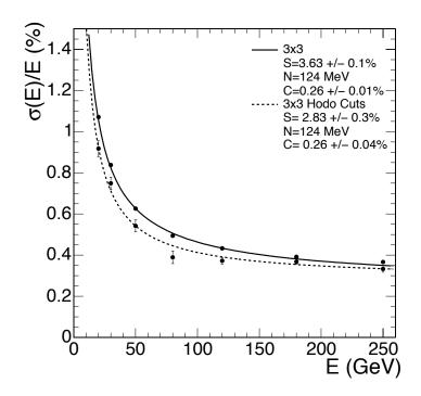
Figure 4.8: ECAL energy resolution as a function of electron energy measured in a  $3 \times 3$  crystal cluster [38].
