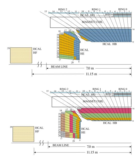
Figure 4.9: Layout of the CMS hadron calorimeter in one r-z quadrant before (top) and after (bottom) the SiPM upgrade. "FEE" indicates the Front End Electronics' locations. Light from layers depicted with the same color are optically added together before reaching the photosensors. The superior photon detection efficiency and response of SiPMs allow for an increased longitudinal granularity with up to 7 depths in HE and 4 depths in HB after the upgrade [49].
