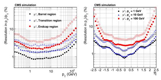
Figure 4.6: Transverse momentum resolution as a function of  $p_{\rm T}$  (left) and  $\eta$  (right) for single, isolated muons in the barrel, transition, and endcap regions of the tracker [47].
