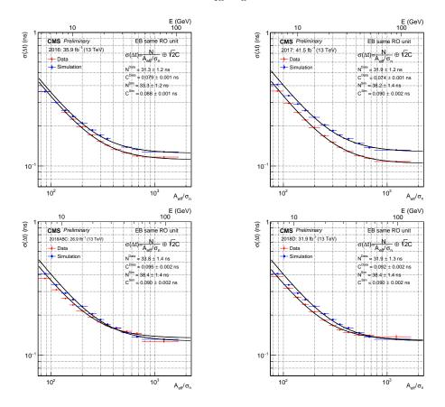
Figure 7.14: Local time resolution of ECAL versus the effective amplitude of the neighboring crystals from the same read-out electronics measured in data and simulation for 2016 (upper left), 2017 (upper right), 2018 eras ABC (lower left), and 2018 era D (lower right). The data in 2018 era D is centrally processed differently by CMS, therefore it requires a separate analysis from 2018 data in previous eras.
