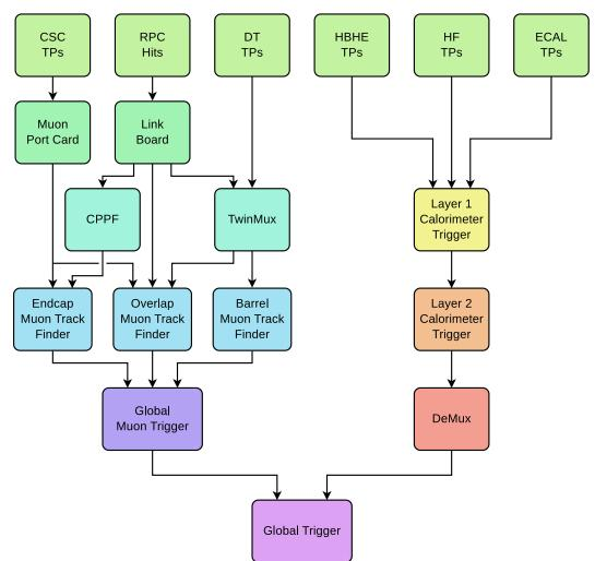
Figure 4.13: Diagram of the L1 trigger system during Run 2 [53].
