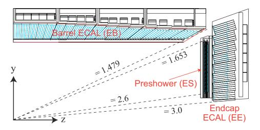
Figure 4.7: Layout of the CMS electromagnetic calorimeter in one r-z quadrant [38].
