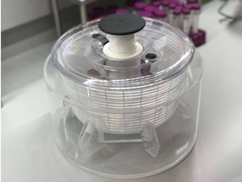
Figure S6. Centrifuge adapted from a salad spinner for concentration tests.
