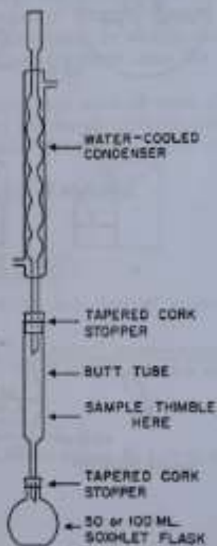
Fig. 1. Butt-type apparatus for oil extraction.
