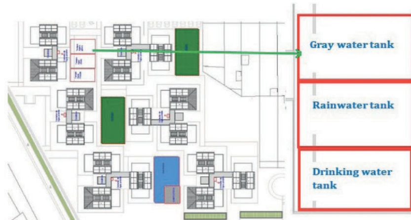
Figure 2.6. Greywater storage for 6 apartment blocks. (zone 1)
