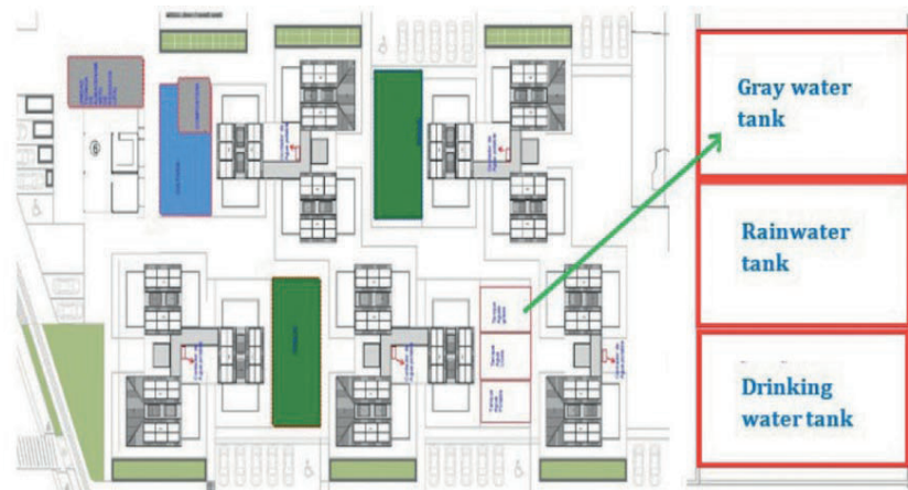
Figure 2.7. Greywater storage for 6 apartment blocks. (zone 2)
