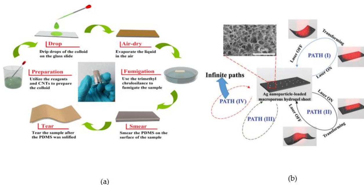
Figure 6. A shape transforming sensor triggered by light, reprinted with permission from [58]. (a) Drop-casting fabrication method, nanocolloid is deposited onto a flexible substrate. (b) Different shape transformations of the sensor depending on the position on which the sensor is exposed to light.
