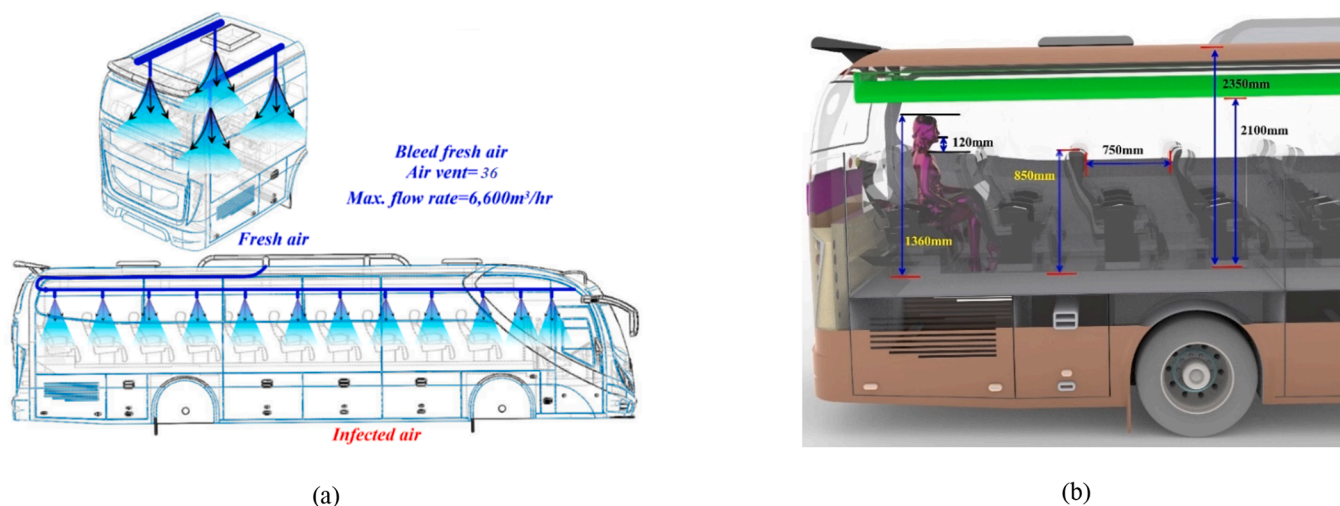
Fig. 1. Ventilation system and the bus geometry a) HVAC duct based on Refs. [32,34], b) location of the sneezing person.
