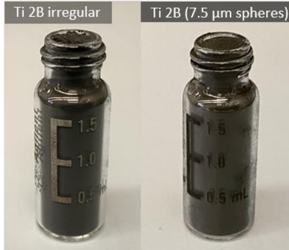
Figure B.2 Glass bottles filled with different powder samples (details on samples). Approximate Ti-2B bulk densities of 11- \mu\text{m} irregular and 7.5- \mu\text{m} spherical powders were respectively 1.93 and 1.80 g/mL. Bulk densities for 18- \mu\text{m} irregular and 93- \mu\text{m} spherical Ti-B powders were 2.22 and 1.77 g/mL, respectively. A slight decrease in bulk density for spherical powders is likely associated with their much greater porosity.
