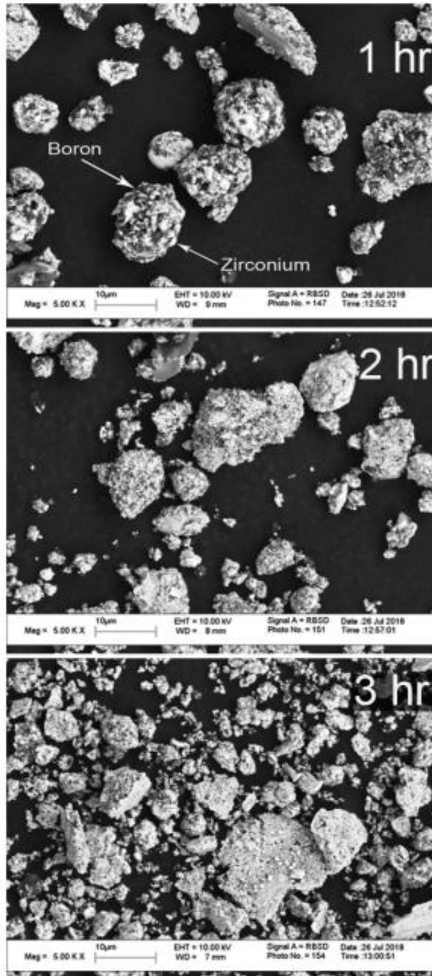
Figure 3.3 Backscattered electron SEM images of prepared composite powders milled for 1 h (top), 2 h (center), and 3 h (bottom).
