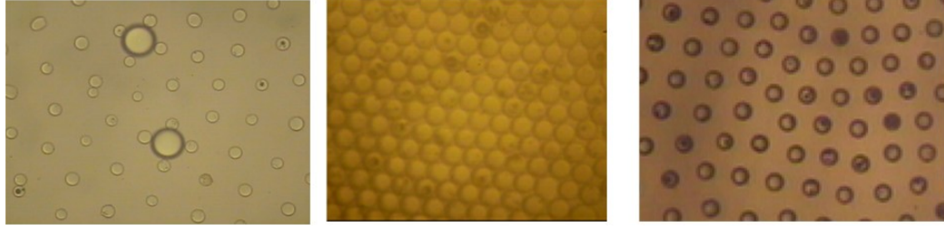
Figure 1.6 Thin films embedded with micron- and nano-sized particles. Monolayers formed by self-assembly under the application of electric field enable us to get different types of particle arrangements with adjustable lattice spacing.
