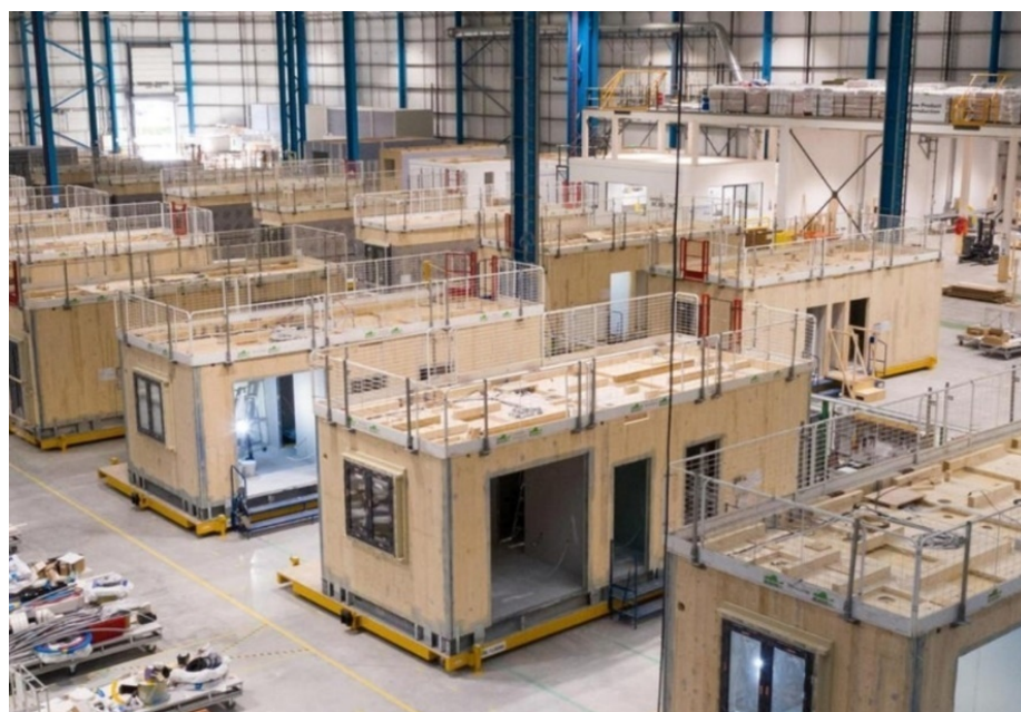
Figure 1. Prefabricated modules in a factory [14].
