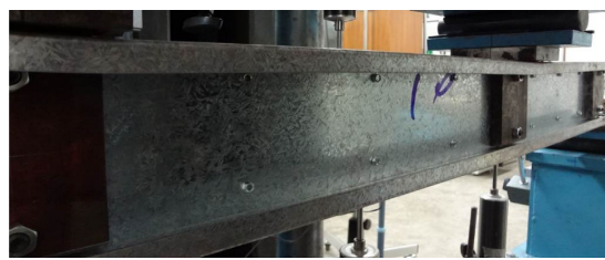
(a) Failure mode of OT1.9-136-S150 [47]
