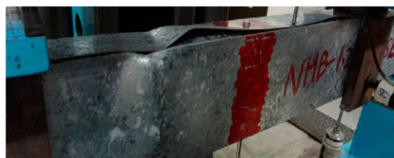
(c) Failure mode of CT1.2-136-S300 [47]
