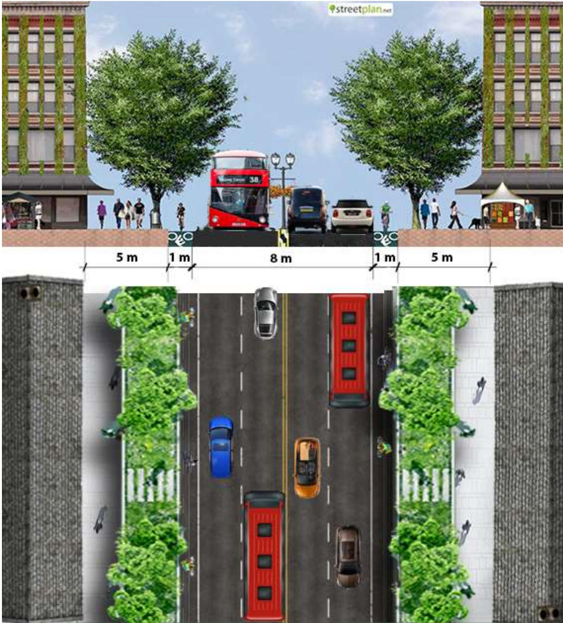
Figure 7-2 Street 50% Trees with 25% Living Facade, on top is street section, while in bottom is street Elevation (Author)
