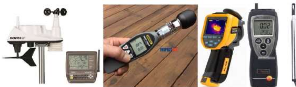
Figure 5-2 Used Equipment, on left Weather station, then Black globe thermometer, then Thermal imaging camera and last equipment is Anemometer (Willmott, 1981)
