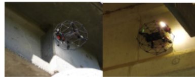
Elios 2 during inspection
