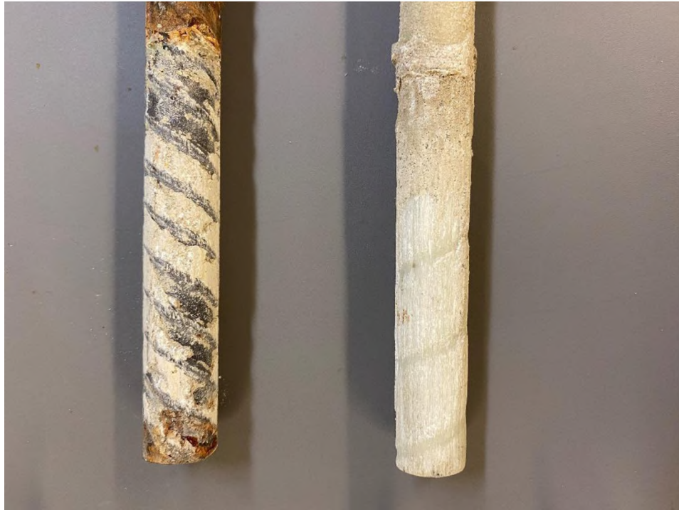
Figure 3. GFRP bar after pullout test
