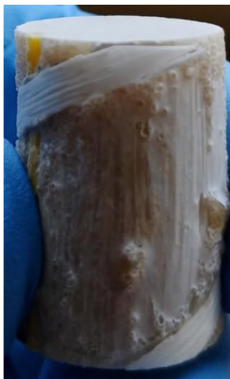
Figure 4. Part of the helical wrap fell off of a bar from the Cuyahoga Bridge during 50° C (122° F) water absorption testing
