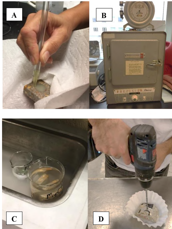
Figure 7. Preparations of Specimens: (A) air drying, (B) oven drying, (C) sonic bath, (D) drilling to get concrete powder
