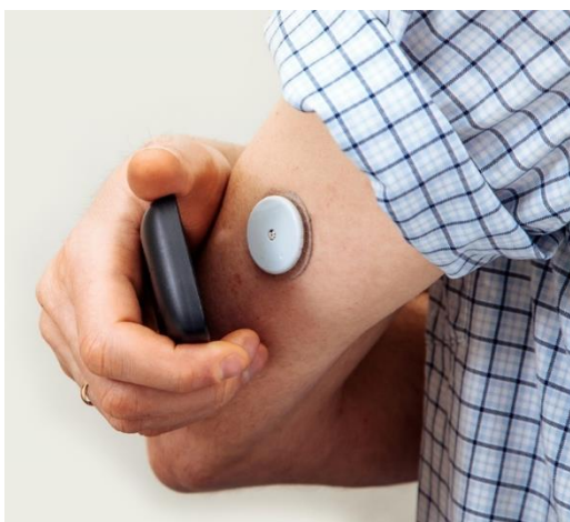
Figure 1.16. Prototype of continuous glucose monitoring system.
