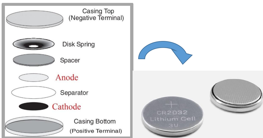
Figure 1.7. Coin cell structure.
