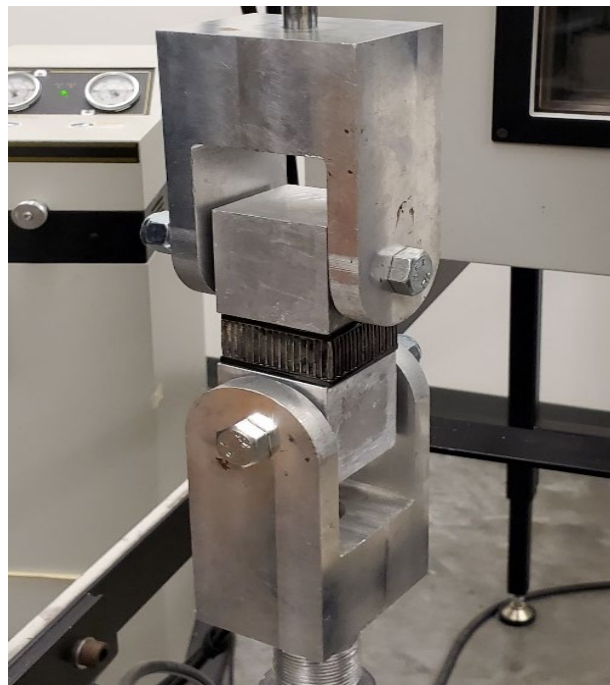
Figure 7. The setup of the flatwise tension test
