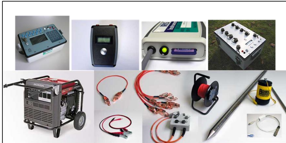
Figure 5.2 Elrec Lite instruments were using of SP survey, IRIS Company, France.
