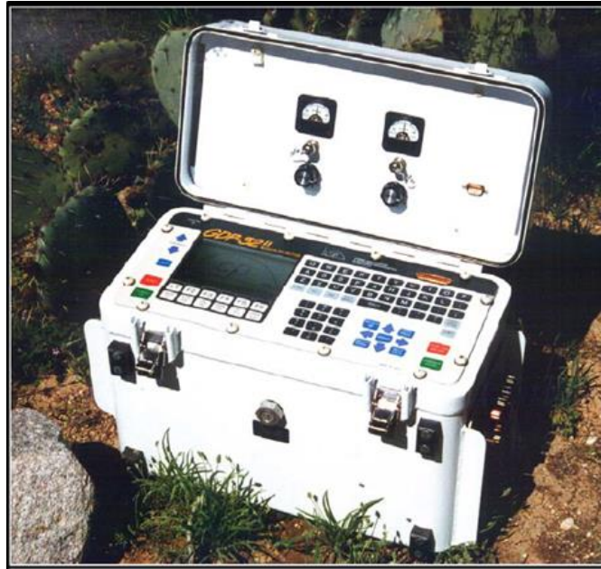
Figure 5.8 GDP-32 receiver used for TDEM survey, A Zonge.
