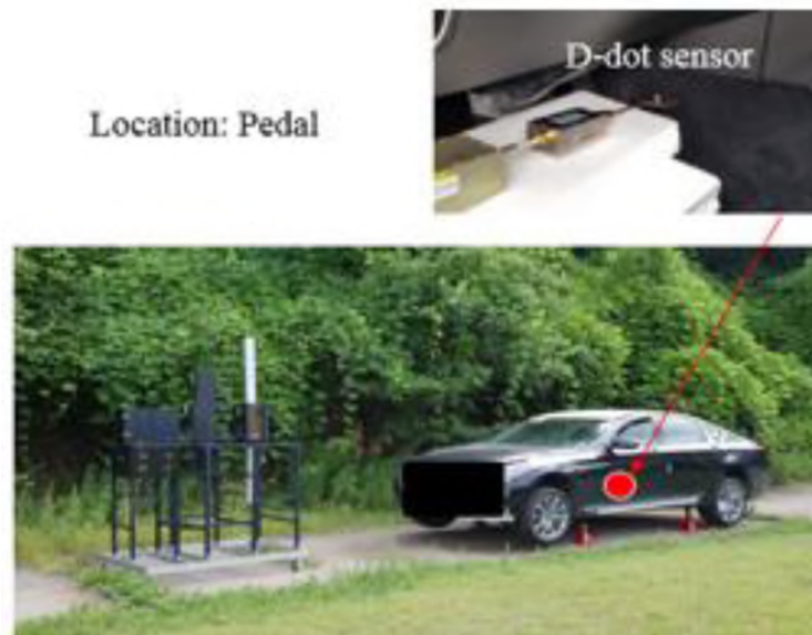
(b) IEMI measurement setup
