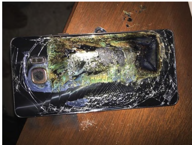
Figure 1. Samsung Galaxy Note7 battery explosion [2]
