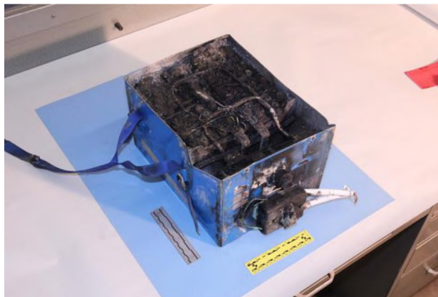
Figure 2. Boeing 787 Li-ion battery explosion [3]
