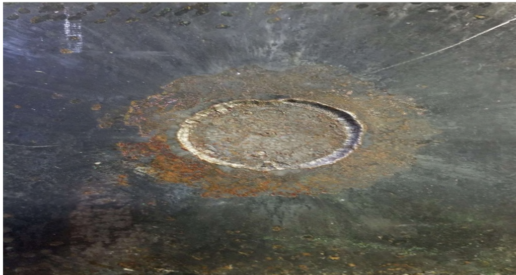
Figure 2.3. Example of a Plate Dent crater on a witness plate to analyze an explosive's brisance cratering abilities.
