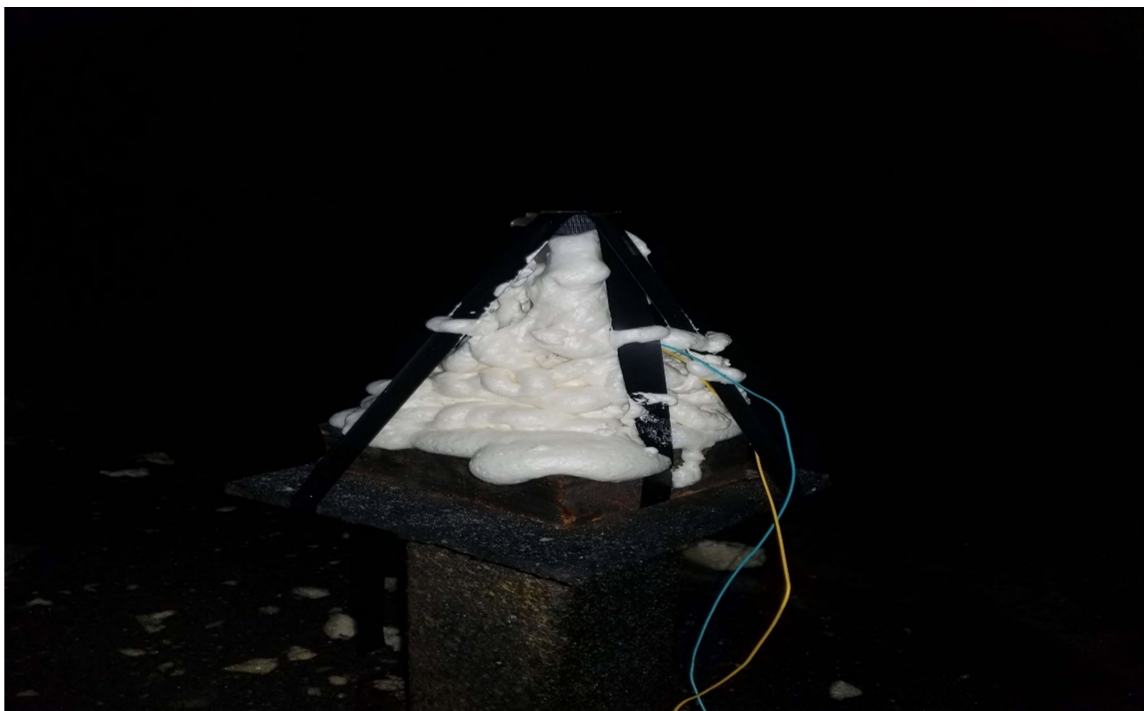
Figure 2.4. Confinement test of TexPak 10-minute foam cure time.
