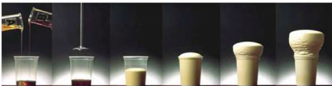
Figure 1.21. A two-part liquid foam was combined and stirred to demonstrate the expanding reaction of polyurethane foam (Carpenter, 2011).
