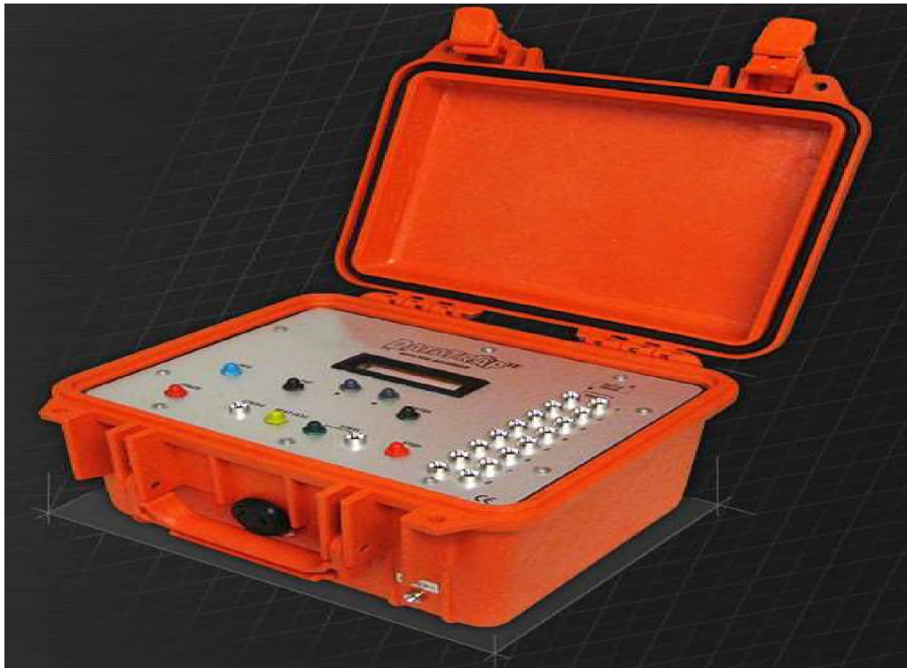
Figure 1.16. Data Acquisition System (DAS) unit manufactured by MREL used for data collection while testing (MREL Group of Companies Limited, 2021).
