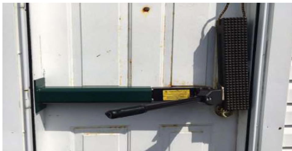
Figure 1.4. A hydraulic breach tool being used to expand a door frame outward to the point of breaking to allow entry into the building (Hansen, 2017).
