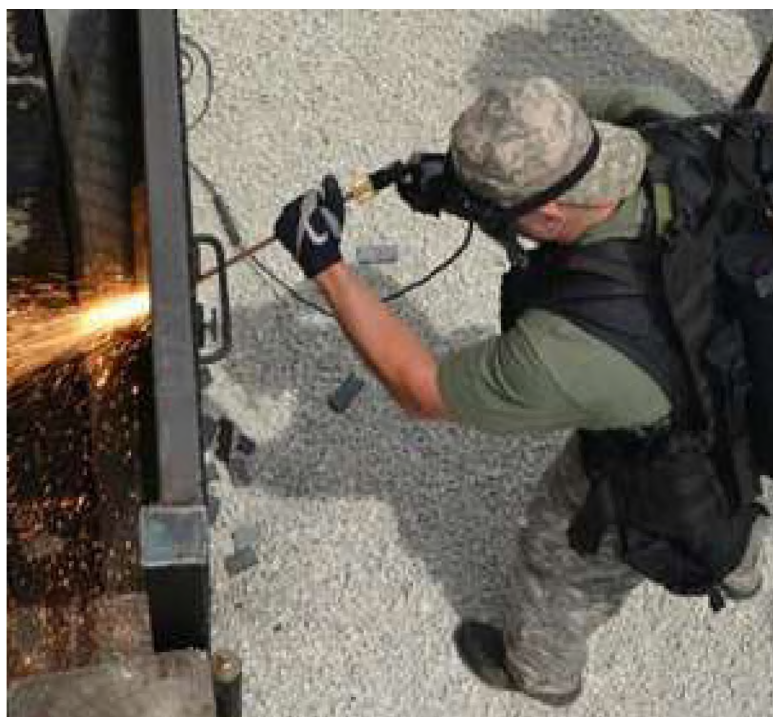
Figure 1.3. A thermal breach being performed using an exothermic torch to cut a metal door handle (Cantrell, 2020).
