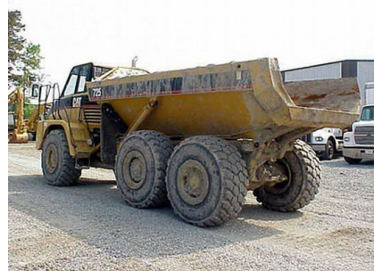
Figure 9. A CAT 725 articulated truck.
