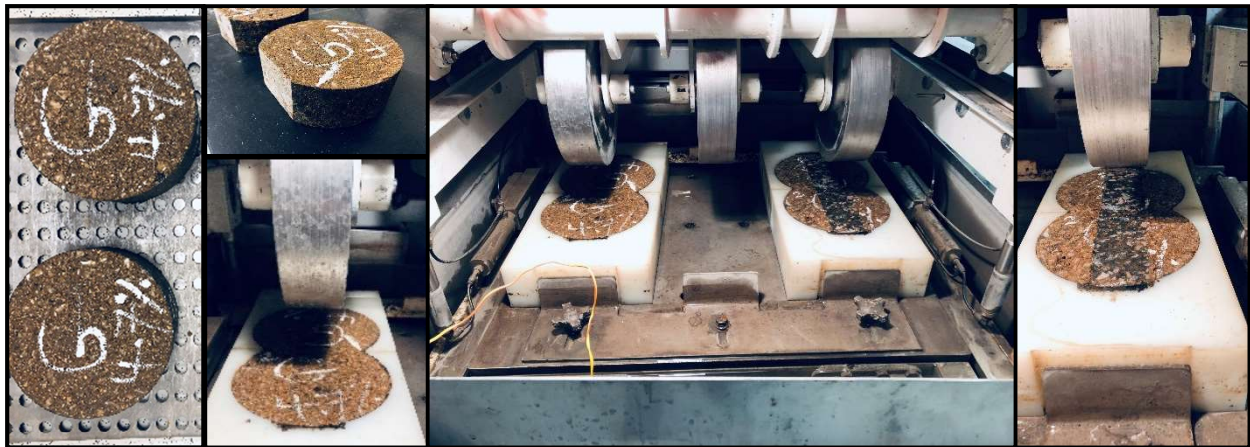
Figure 6. Technical steps from the HWT test procedures.
