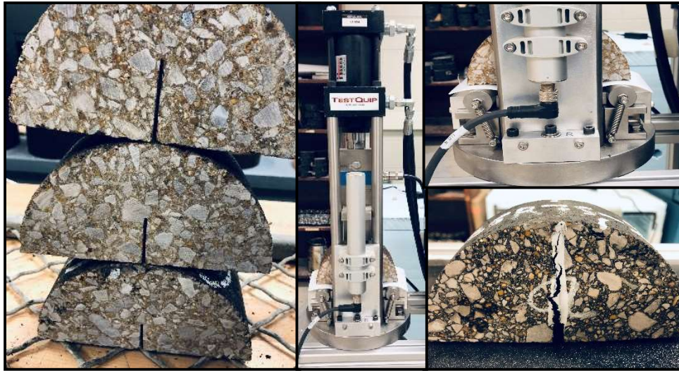
Figure 7. Technical steps from the SCB test procedures.
