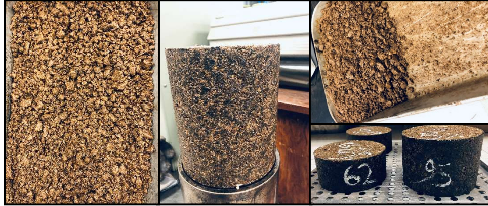
Figure 3. Neat guayule mixture (G-Mix): loose and compacted.
