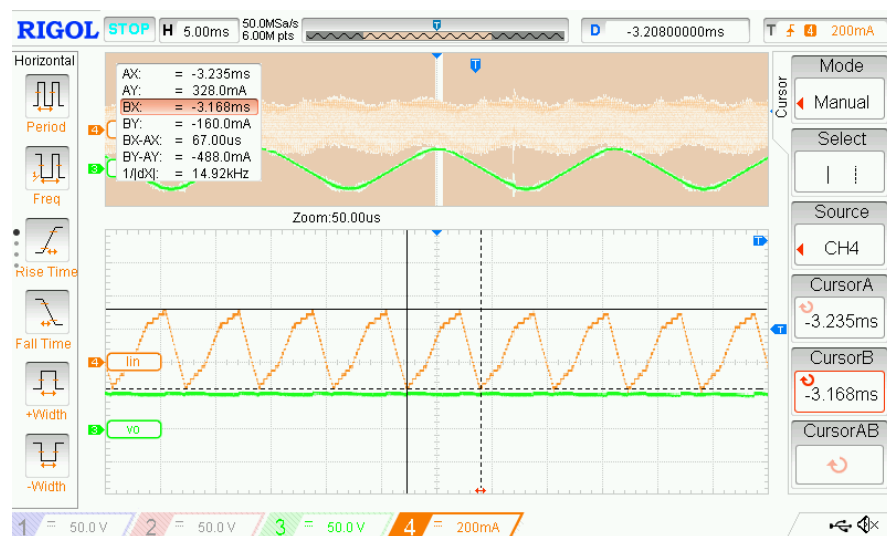
Figure 29. Measurement of output voltage and input current. The ripple in the current waveform demonstrates the 15 kHz switching frequency.
