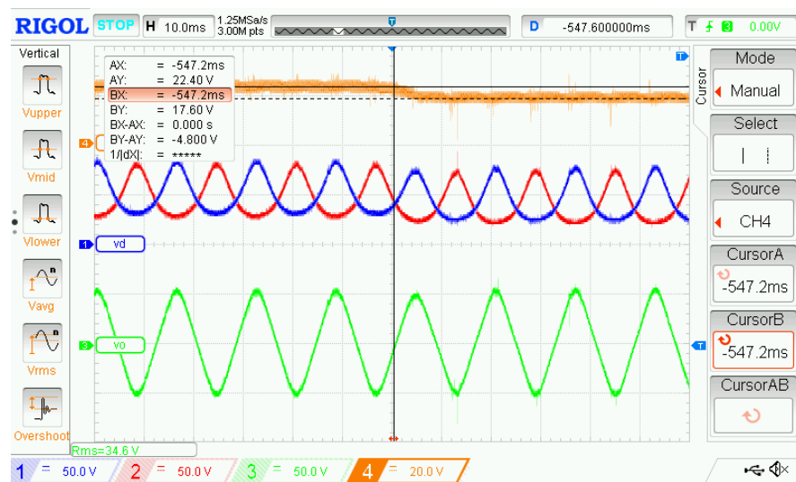
Figure 24. Measurement of capacitor voltages and voltage across the load when the supply is changed.
