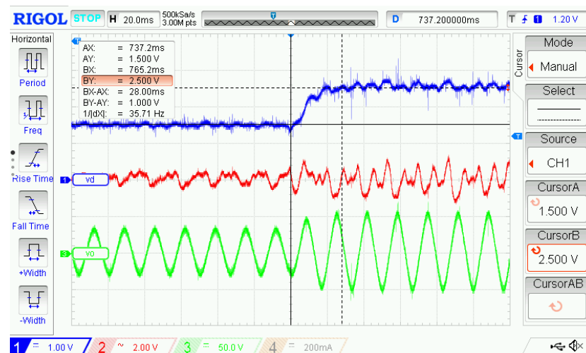
Figure 23. Measurement of output voltage and dq axis voltages as the reference is changed.
