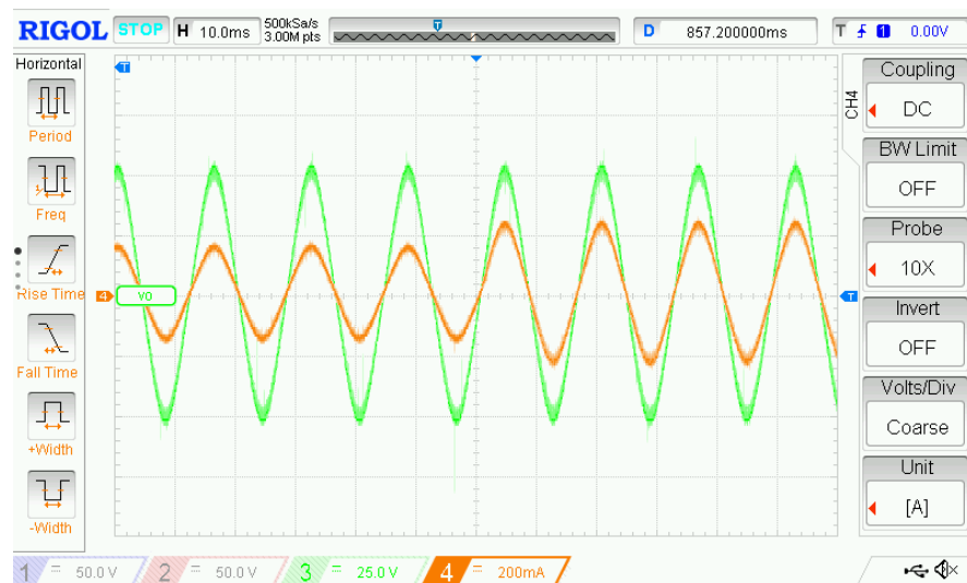
Figure 25. Measurement of load voltage and load current due to a step change in resistive load.
