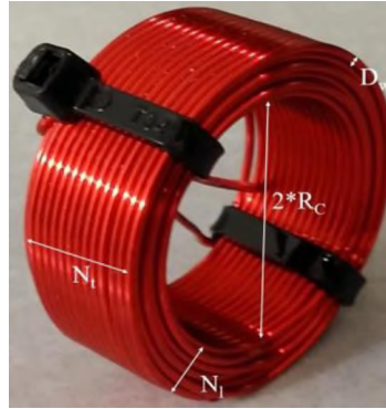
Figure 5. Photo of a typical coil illustrating the parameter definition of the coil model.
