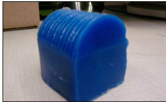
Fig. 3: Machined Semi-Cylindrical Geometry
