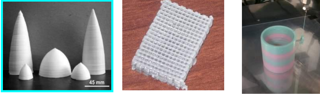
Figure 2. Sample parts fabricated by the FEF process
