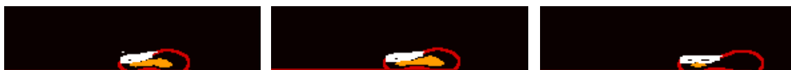
Figure 14. Melt pool (white) solidus zone (yellow) and deposit boundary (red), left to right progression in deposition
