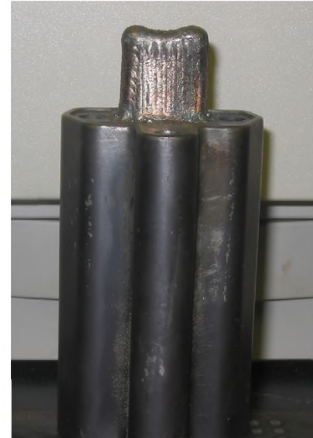
Figure 14. Repaired Core - via Automated Part Repair
