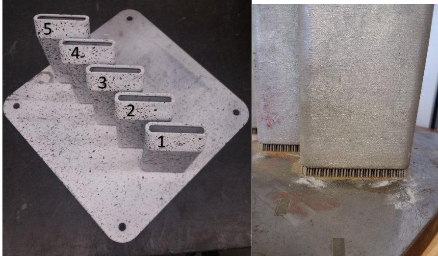
Figure 3 - 1st AM Build test – 5 chimneys
