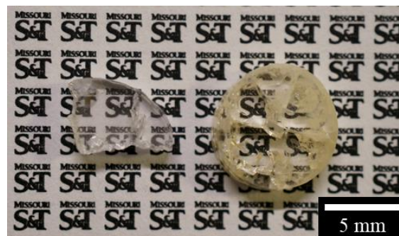
Figure 4. Typical printed pure spinel samples after cross-sectioning and polishing. Obvious cracking is observed with part of a cracked pure spinel sample also shown.
