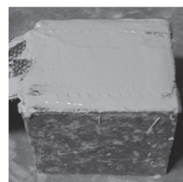
(f) Brushing the surface adhesive.
