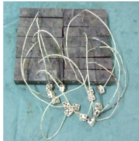
Fig. 14 Specimens with thermocouples.
