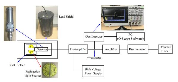
Figure 2. A schematic of the experimental setup for the radiation counting system.
