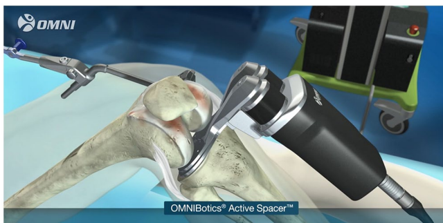
Fig. 6 BalanceBot robotic soft tissue balancer (formerly OMNIBotics active spacer).
