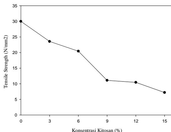
**Gambar 4.** Sifat mekanis (*Tensile Strength*) hidrogel fim PVA/Kitosan
