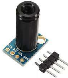
Gambar 1 Sensor IR MLX90614 (Systems, 2019)
