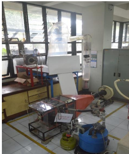
Gambar 3.1 Instalasi peralatan fluidized bed coal dryer
