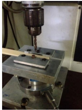
Figure 9. GFRP drilling process using dynamometer Kistler.
