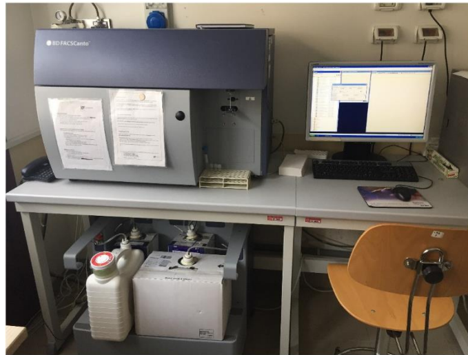
Figure 15: BD FACS Canto machine, instrument used to perform Flow Cytometry analysis. (Own photo).
