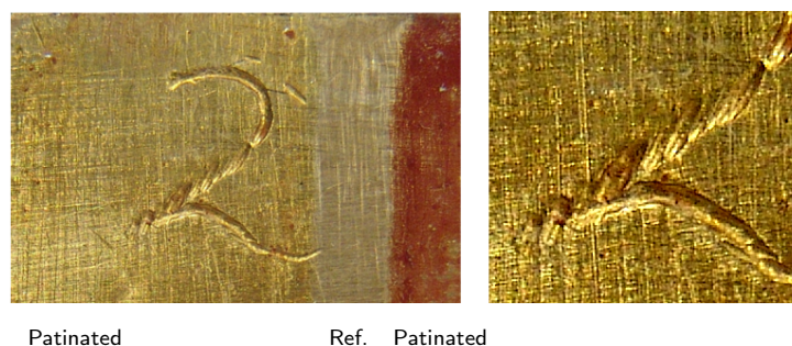
Figure 5.6: Photograph of patinated bronze mock-up with engraved the number “2” (see Fig. 5.7 for precise dimensions). Two different patination processes have been used while a stripe between them has been left as reference (left). Detail of the engraver grooves and the material scratches (right).
