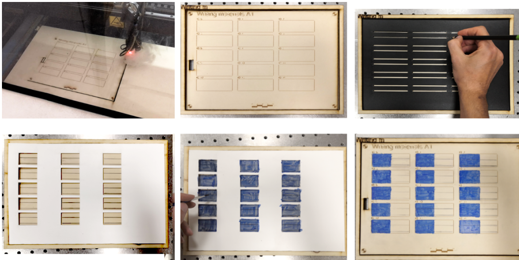
Figure 2.3: The creation of the samples collection using an industrial laser cutter and the masks for easing the application of the layers. From left to right, on the first row: cutting of the panel, resulting panel with the border and positioning of the first mask. From left to right on the second row: positioning of the second mask, painting of the areas and final result.
