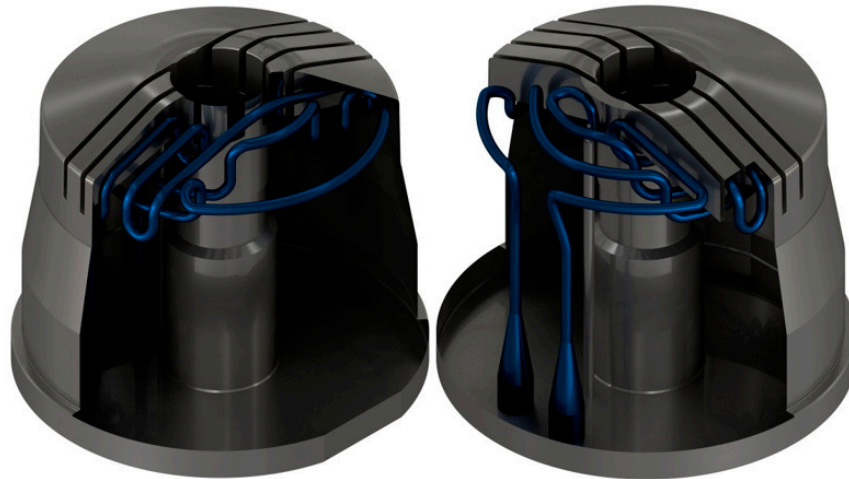
Figure 18. 3D sectional model of the injection molding tool from two perspectives.
