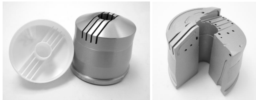
Figure 21. The final manufactured injection molding tool with the principle part ( left ) and sectional part exhibiting the integrated cooling channels ( right ).
