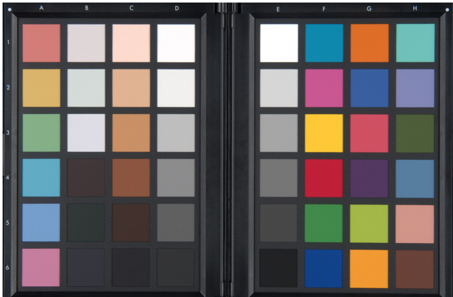
Figure A.1. Test scene used for noise parameter calibration.
