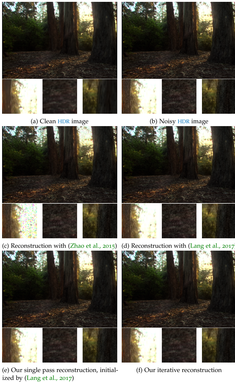
Figure 6.2. Comparison of reconstruction results for an image from the Debevec dataset. A 16 bit HDR camera is to be reconstructed from 10 bit modulo images. Reconstructed images are shown after tone mapping with the operator of Drago et al. (2003).
