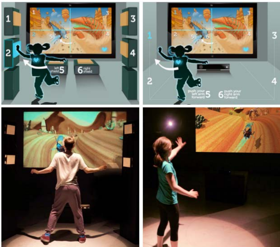
Figure 6: Prototypical state of two motion-based controller setups (left: full-body motion controller; right: Kinect) of the adaptive exergame Plunder Planet.
