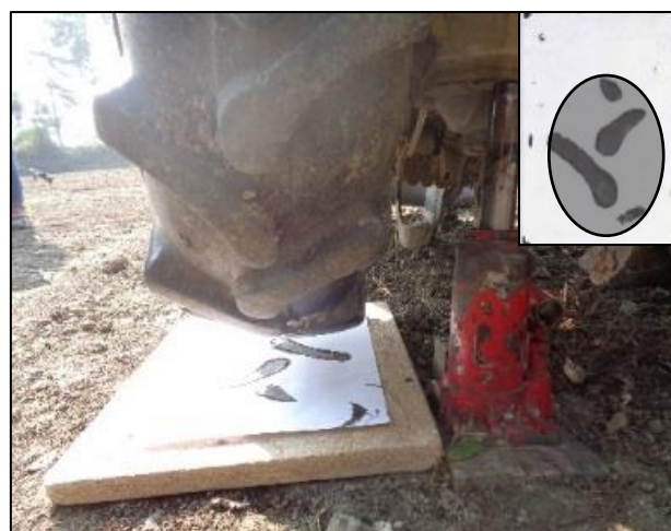
Figure 4.1 Determination of tyre soil contact area by taking an impression of the tyre on a sheet of paper. Inset is the impression of the tyre.
