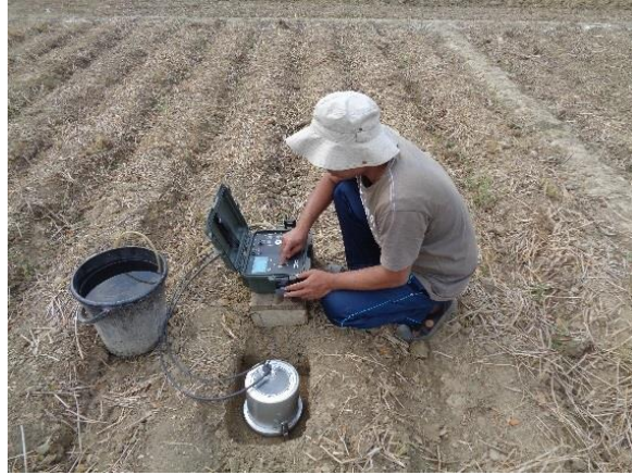
Figure 3.5 Field measurement of saturated hydraulic conductivity with a constant head digital infiltrometer (Meter group, USA). Picture showing measurements in the furrows.
