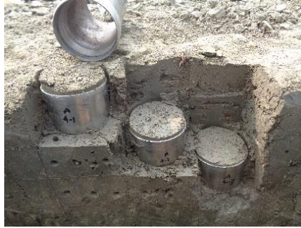
Figure 4.3 Sample core collection from three depths (0-5 cm, 5-10 cm and 10-15 cm) of a trench for bulk density and penetration resistance measurements at Digram. For Alipur the soil sampling increments were 0-5, 8-13, and 10-15 cm.
