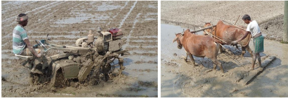
Figure 2.1 Soil puddling by a two-wheel tractor and levelling for conventional transplanting of rice.
