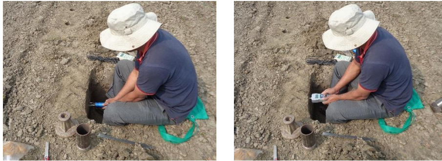
Figure 4.4 Measurements of soil water content and penetration resistance in the trench after wheel compaction operations at Alipur in 2015.
