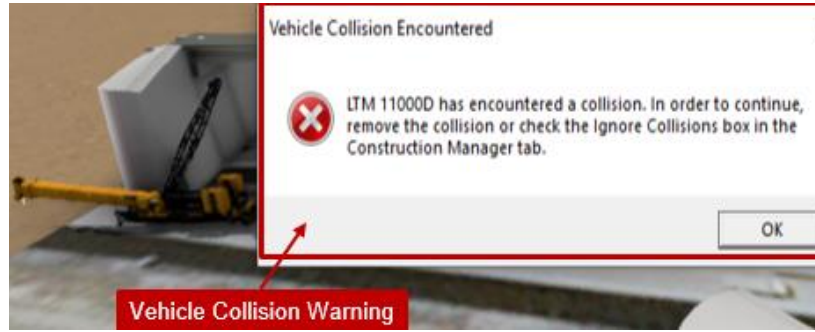
Figure 5.19: Equipment conflict warning
