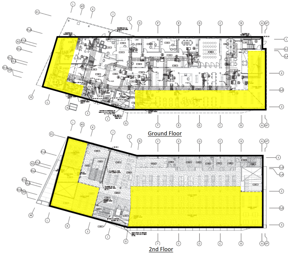
Figure 4.2: Varennes library plan highlighting areas supplementary served by a hydronic radiant slab circuit.
