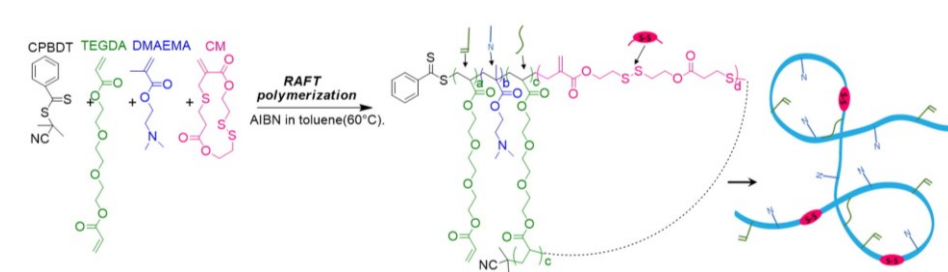
Figure 2.7. Synthesis of backbone-degradable single-chain cyclized polymer poly(DMAEMA-co-MDTD-co-TEGDA) by RAFT polymerization. 103
