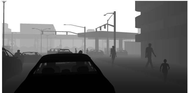
(b) Depth frame containing pixel-wise distance information
