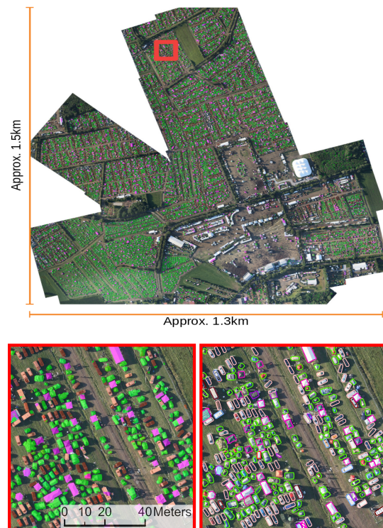
Figure 1. Illustration of a sample result from DLR-AerialTent dataset with pixel- and instance-wise segmentation using aerial imagery of a music festival in 2013 in Germany with 9cm/px GSD. The red outlined area represents a sample from the test set.
